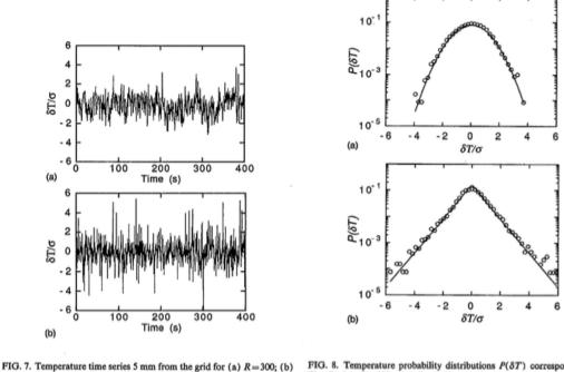
R = 1850. The temperature is expressed in units of the standard deviation. Frequent large excursions from the mean are seen in case (b).
