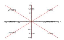
Figure 4: Bifurcation diagram (Union Jack)! For r > 0, the branches are (from bottom), stable, unstable, stable. For r < 0, the branches are unstable, stable, unstable. For r=0, all values of x are stable (vertical line).
