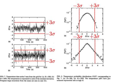
Figure 1: (a, left) Timeseries of temperature differences from mean value for R=300 run, normalized by its standard deviation. (b, left) Normalized timeseries from R=1850 run. (a, right) Probability density function (with normalized histogram) of temperature differences for R=300. (b, right) PDF and histogram for for R=1850.
