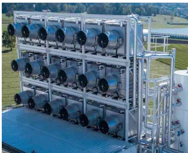
Figure 2: Climeworks AG facility near Zurich, Switzerland, a DACS facility. Constructed in 2017 atop a heat recovery plant, this device is expected to capture 900 tonnes of CO 2 per year at a cost of over $1000/t CO 2 . Rather than being stored, the CO 2 is pumped into a nearby greenhouse [10].
