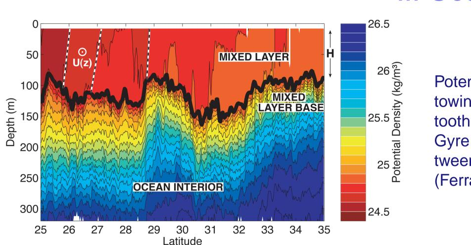
The ocean mixed layer (ML) is a layer of weak stratification in the upper 100 m overlying the more stratified thermocline. The ML is not horizontally homogeneous: there are numerous lateral density gradients. ADCP measurements collected during the same campaign confirm that the lateral density gradients are in geostrophic balance with a sheared velocity  $U_z$  as schematized here.
