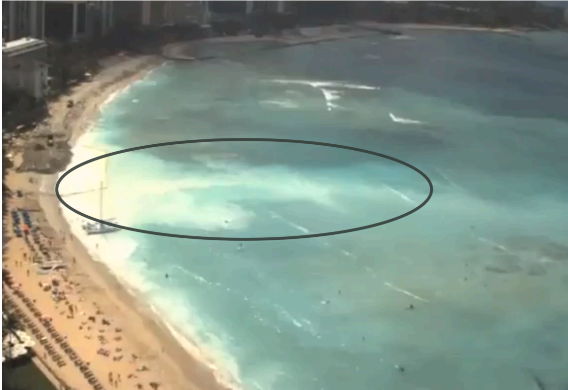
Figure 3: Image from video footage of sand replenishment project. The circle marks the location of the rip current highlighted by the sand.
